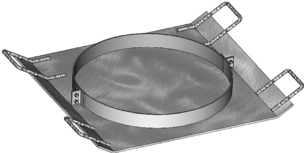
FIG. X1.2 Simple Steel Form With Rigid Base and Handles for Transport and Handling
