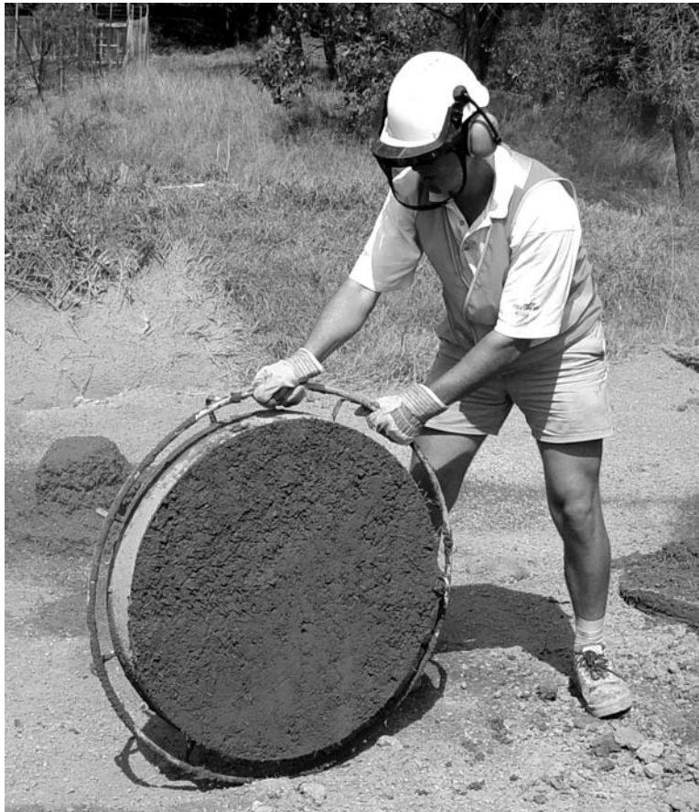
FIG. X1.4 Rolling Steel Form after Specimen Has Gained Sufficient Strength to Withstand Damage
