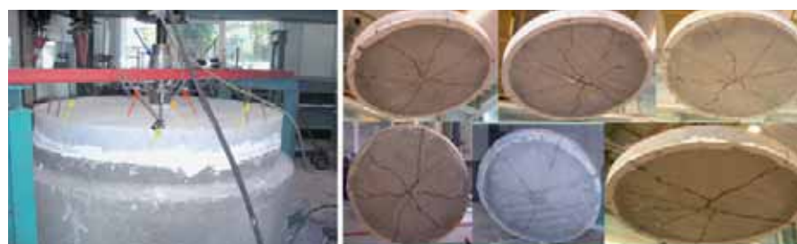
Figure 6: Round slab test set-up (left) and typical fan pattern cracking (right).
