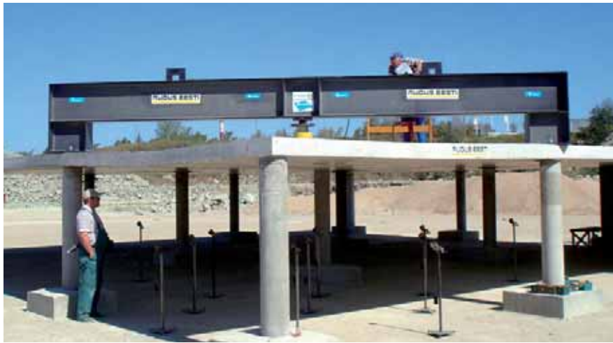
Figure 3: Point loading of the corner span of the Tallinn test slab.
